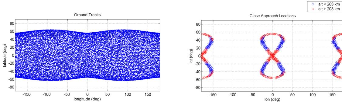
**Figure 10: Long term n body ephemeris propagation of example 8:35 science orbit: full ground tracks (left) and close approaches (right)**
