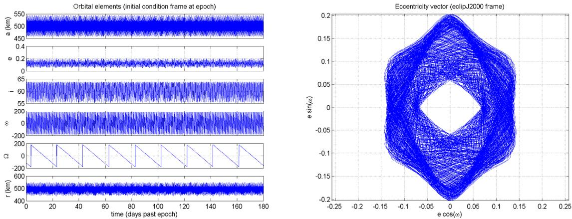
**Figure 9: Long term n body ephemeris propagation of example 8:35 science orbit: orbital elements evolution (left) and full eccentricity vector repeat path (right)**
