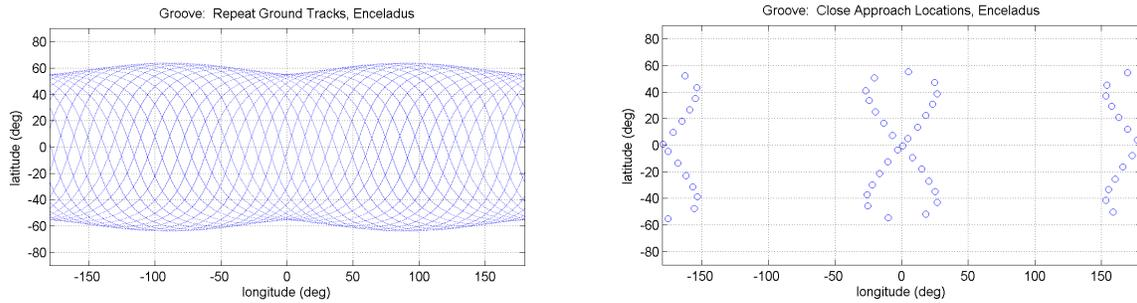
**Figure 5: One period of example 8:35 science orbit: full ground tracks (left) and close approaches (right)**
