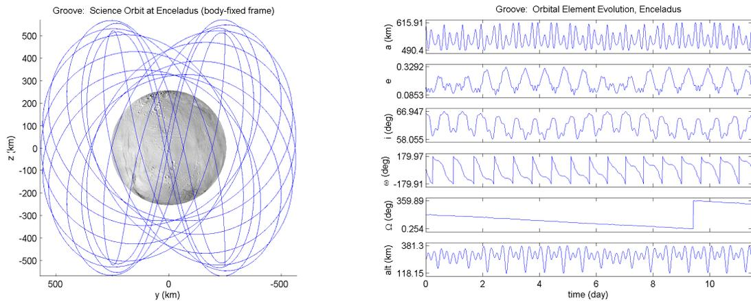
**Figure 8: One period of example 9:35 science orbit: trajectory (left) and orbital elements (right)**
