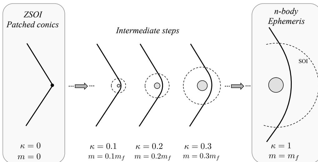
**Figure 1:** Schematic of the continuation method preserving flyby geometry and turning angle
