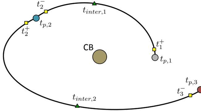
**Figure 4:** Patch times (squares) and intermediate times (triangles) for three target bodies
