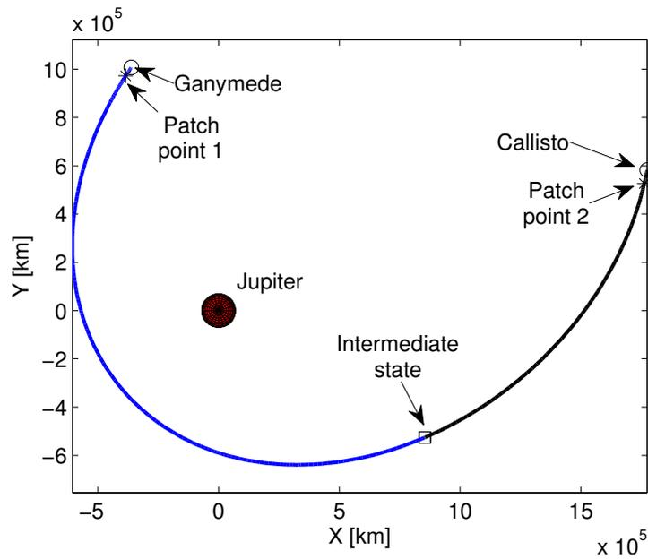
**Figure 5:** Converged transfer from Ganymede to Callisto
