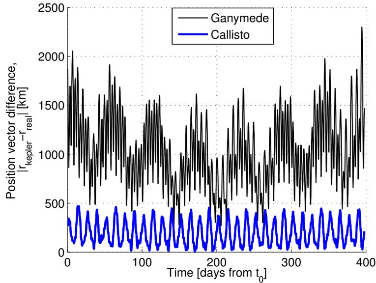
**Figure 3:** Variation in orbital position between the Keplerian and real ephemerides, demonstrating good ephemeris matching
