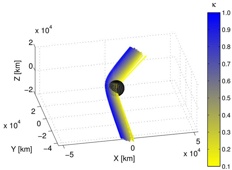
Figure 10: Successive iterations of the first flyby trajectory at Venus. Venus is shown at its final (actual) radius.
